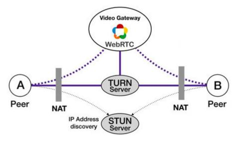
The STUN server basically sends 2 types of responses: successful or error, every response has a list of attributes which contains information about binding IP address, error code, reason of error...
