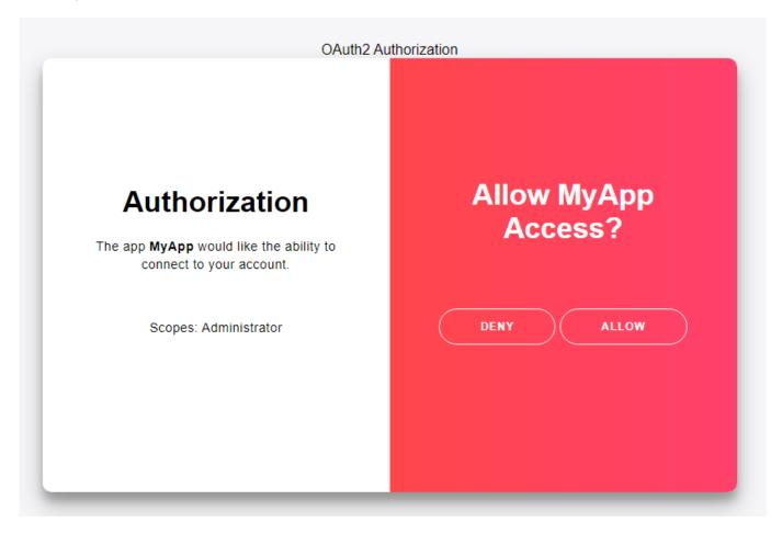
If the user Allows the access, a login form will be shown where the user must set the Username and Password. This data will be received OnOAuth2Authentication event, so you must validate than the user/password is correct and if it is, then set Authenticated parameter to true.
